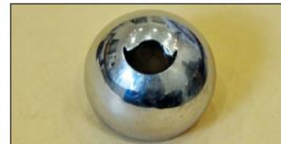
Figure: Metal hip prostheses causing cobalt intoxication. Removed metal head with hole due to severe metal ion.
